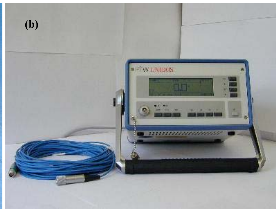
Figure 1 – Circulating instrument consisting on: (figure a) ionisation chamber PTW type 23361 with a build-up cap for the energy of ^{137}\text{Cs} and ^{60}\text{Co} gamma radiations; (figure b) associated measuring assembly PTW UNIDOS type 10002 with a 20 m. long extension cable to connect the detector and the measuring assembly.
