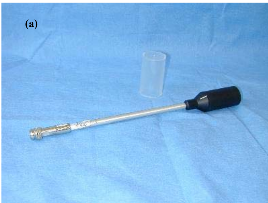
Figure 1 – Circulating instrument consisting on: (figure a) ionisation chamber PTW type 23361 with a build-up cap for the energy of ^{137}\text{Cs} and ^{60}\text{Co} gamma radiations; (figure b) associated measuring assembly PTW UNIDOS type 10002 with a 20 m. long extension cable to connect the detector and the measuring assembly.
